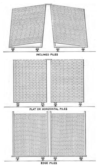
Fig. 98.—Methods of piling lumber for kiln drying.
